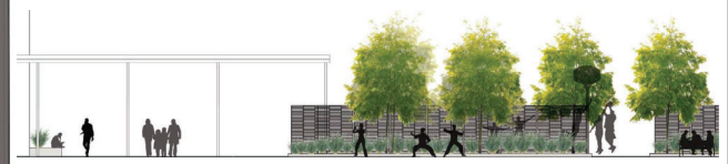
Metal "Bamboo" Screen Elevation The screen provides a separation between passive and active activity areas and protects passive users from basketballs.
