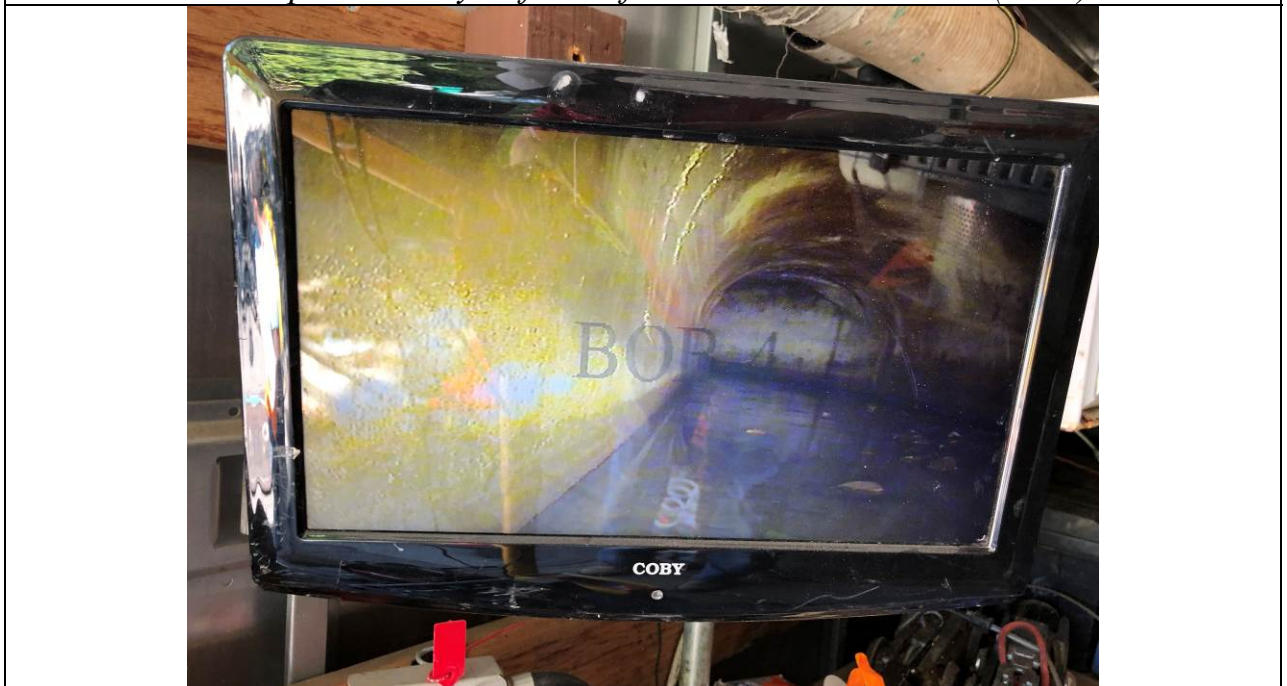
Work Item #1 - Photo 3 Robot "BOB-4" with camera. TV view of the poured concrete 100 plus year-old culvert directly under 901 Trestle Glen Rd (2019). Install three grade beams to further separate the house from the culvert 17-ft below the house grade level.
