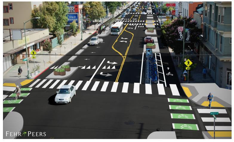
**Option 4:** Enhanced Buffered Bike Lanes (Conventional bike lanes with painted buffers between the bike lane and moving vehicles and between the bike lane and parked cars, concrete bus boarding islands, and two protected intersections)
