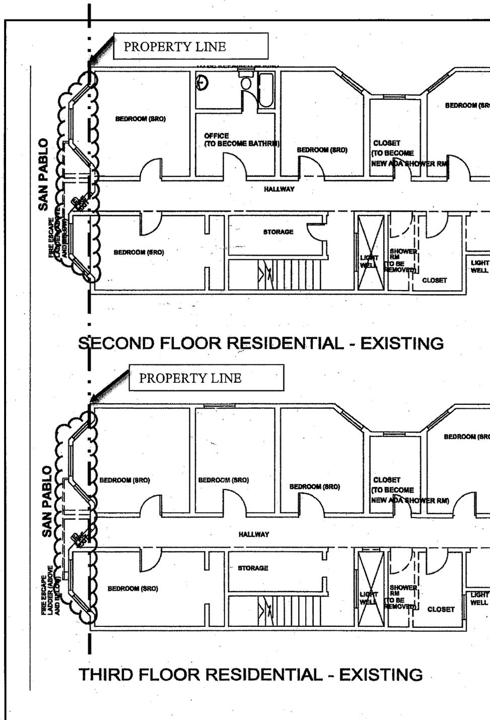
Three (3) existing outward swinging doors encroach approximately three (3) feet each in the Public Right-of-Way. Portions of existing building encroach approximately three and a half (3.5) feet with approximately eighty (80) square feet of area encroaching into the Public Right-of-Way.
