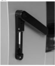
Figure 2. Complete insertion of EZ1 Card. The EZ1 Card must be completely inserted before the EZ1 instrument is switched on.
