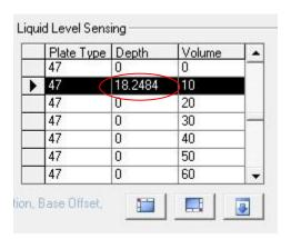
Figure 9-99 Check (Offset Calculator) and Enter New Depth Offset for 10uL Volume
