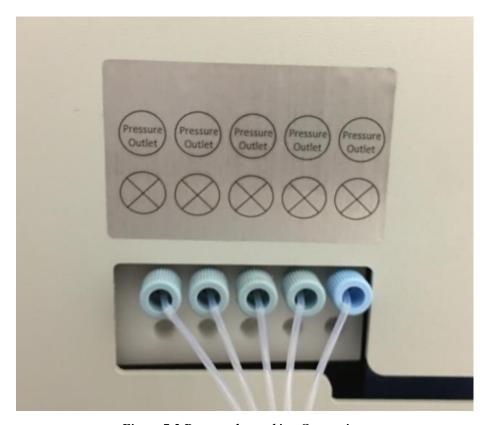
Figure 7-2 Reagent drop tubing Connections
