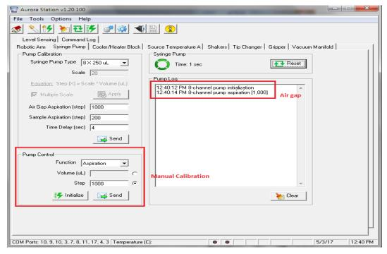
Figure 9-47 Syringe Pump Calibration-Manual mode
