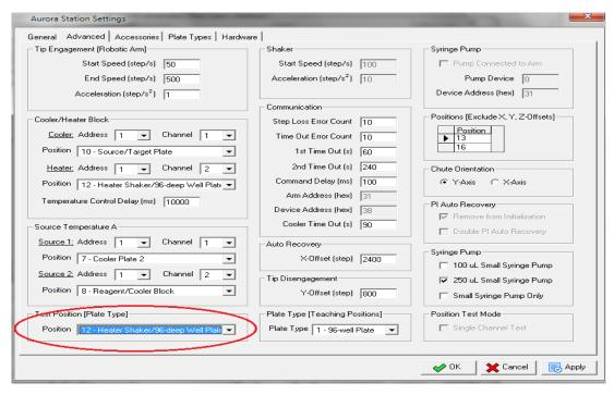
Figure 9-26 Reagent Drop pin position testing-test position selection
