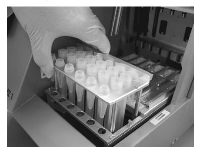
Ensure that the tips, tip holders, and tip rack are correctly positioned on the worktable.
