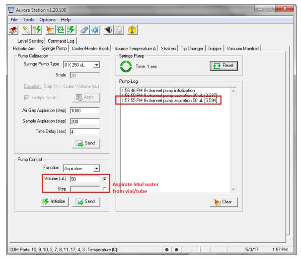
Figure 9-56 Syringe Pump –Aspirate 50µL volume
