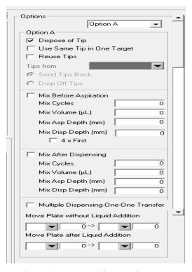
Figure 11-10 Advanced Reagent Addition Tab—Option A parameters
