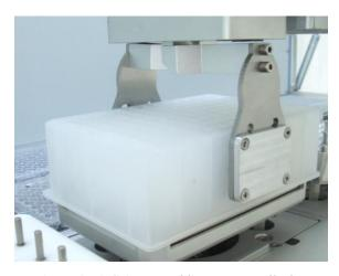
Figure 9-63 Gripper Holding Deep Well Plate
