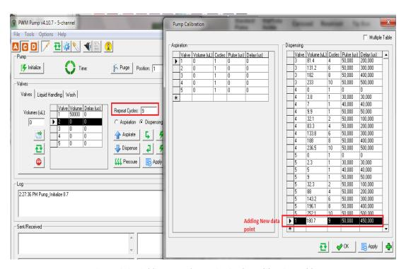
Figure 9-37 Adding new data point in the calibration table
