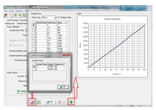
Figure 9-50 Syringe Pump Calibration-Graph & Scale
