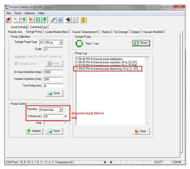
Figure 9-57 Syringe Pump –Dispense back to vial 10µL
