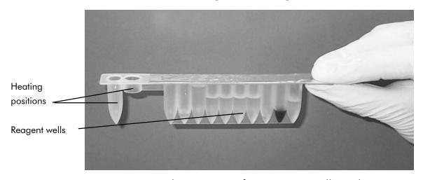
A reagent cartridge consists of 10 reagent wells and 2 heating positions. One heating position is a well, the other is a slot that can accept a tube.
