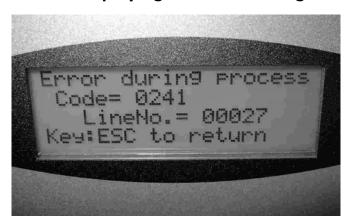
The second line of the error message gives the error code (see list below). The third line indicates the line number of the protocol at which the error occurred.
