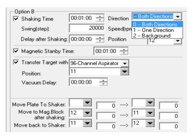
Figure 11-12 Advanced Reagent Addition Tab—Option B parameters
