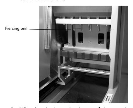
5. Wipe the piercing unit using a soft tissue moistened with distilled water.
