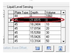
Figure 9-81 Check Depth Offset (Calculator) at 10 µL with Depth Value under Aurora Station Plate
