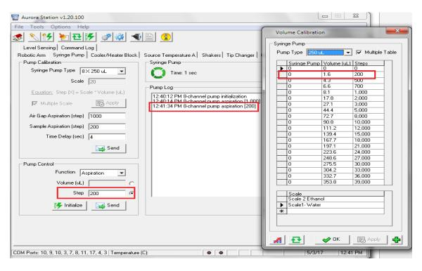
Figure 9-48 Syringe Pump Calibration-Aspirate volume
