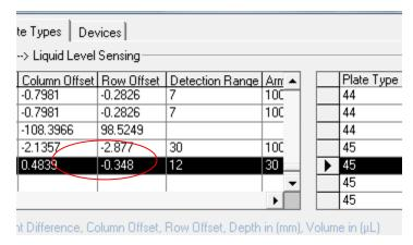
Figure 9-97 Enter Signal Difference under Aurora Station Plate Types Tab Detection Range Field
