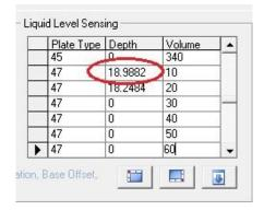
Figure 9-101 Check (Offset Calculator) and Enter New Depth Offset for 0uL Volume
