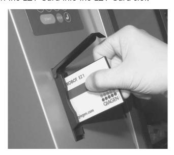
Orientate the card so that the picture faces to the left and the triangle symbol is at the bottom.
