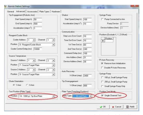
Figure 9-70 Setting the Tip Box Position, Plate Position & single channel mode for Calibration
