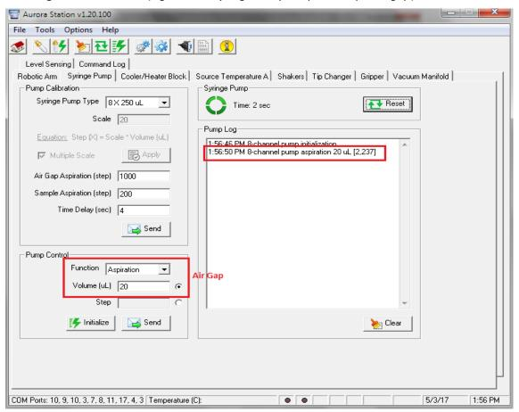
Figure 9-55 Syringe Pump -Aspirate 20µL Air-gap
