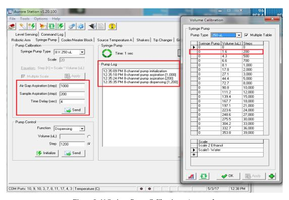
Figure 9-46 Syringe Pump Calibration—Auto mode
