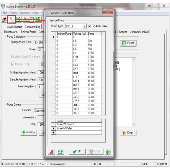
Figure 9-44 Syringe Pump Calibration
