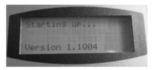
This text indicates that the BioRobot EZ1 DSP is initializing. All motors move to their home positions.
