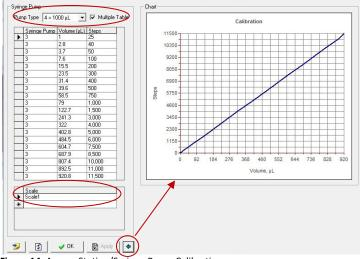
Figure 14: Aurora Station/Syringe Pump Calibration
