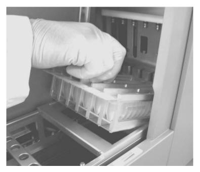
Ensure that the 2 heating positions of each cartridge fit into the heating system.
