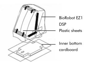
**Note**: Be careful not to damage the surface of the BioRobot EZ1 DSP after removing the plastic sheets.
