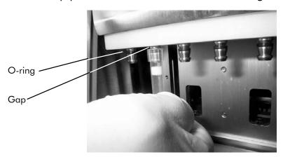
**Note**: The filter-tips should sit flush against the upper white plastic bar if the O-rings are properly greased. There should not be a gap. Excess or insufficient grease can affect the performance of the BioRobot EZ1 DSP.
