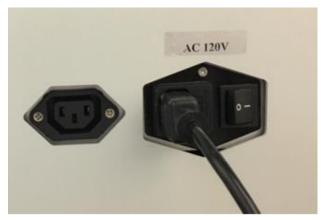
Figure 7-6 VERSA and Vacuum pump Power Connections
