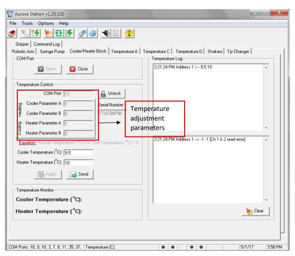
Figure 9-59 Cooler Block Control
