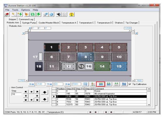
Figure 9-13 Aurora Station- Picking 20ul tip from position #2
