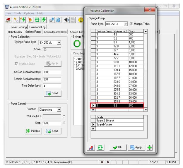
Figure 9-52 Calibration Table New Data Point Entry
