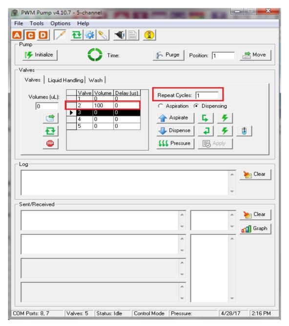
Figure 9-29 PWM pump-Dispense 100ul volume-Pin # 2
