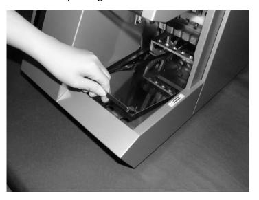
Reverse this procedure to replace the tray. To avoid instrument damage, ensure that the tray is positioned correctly.
