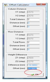
Figure 9-100 Check (Offset Calculator) and Enter New Depth Offset for 0uL Volume
