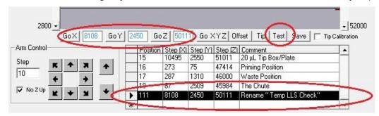
Figure 9-77 Saving Surface Coordinates into Aurora Station Robotic Arm Interface
