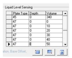
Figure 9-88 Entering New Plate Type Numbers with Corresponding Volumes prior to LLS Calibration Test
