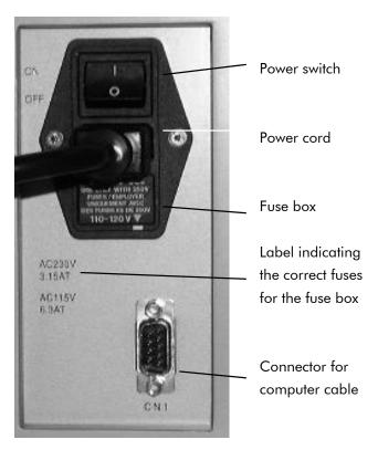
It contains the power switch, the socket for the power cord, the fuse box, and a connector for a computer cable (for service use only).
