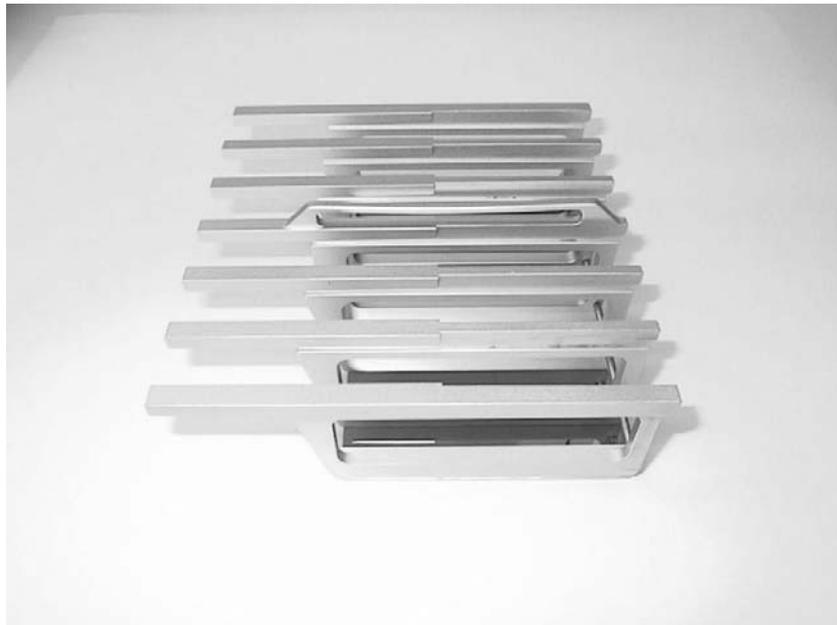
Reagent cartridges are made of polypropylene, contain prefilled reagents, and are available from QIAGEN.
