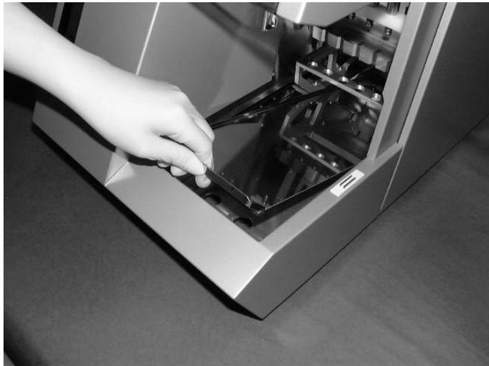
Reverse this procedure to replace the tray. To avoid instrument damage, ensure that the tray is positioned correctly.
