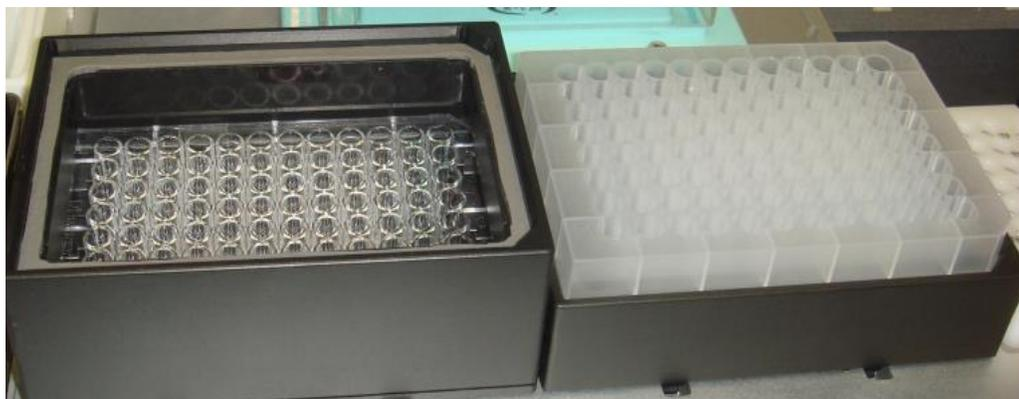
**Figure 9-17 Vacuum Wash & Sample Collection Positions**
