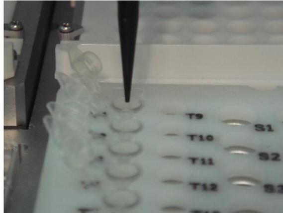
***Figure 9-23 39 Well Reagent cooler Block-Testing T1 Position***
