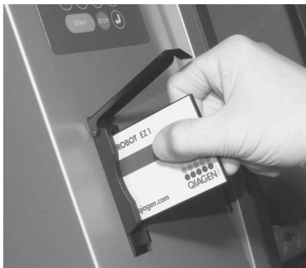
Orientate the card so that the picture faces to the left and the triangle symbol is at the bottom.
