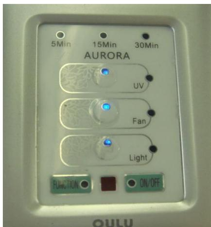
*Figure 12-2 UV/HEPA Bio-Containment Hood—Control Panel*
