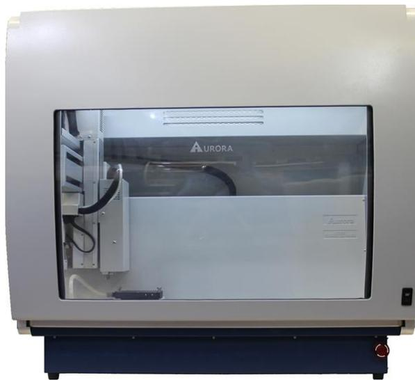
*Figure 12-1 UV/HEPA Bio-Containment Hood*
