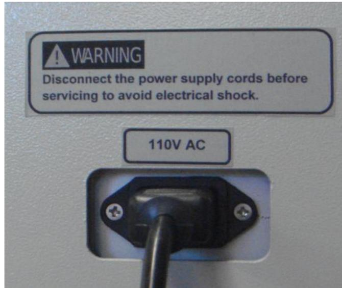
*Figure 7-4 UV/HEPA power cable connection*
