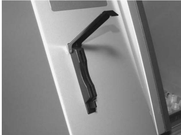
It is extremely important that the EZ1 Card is completely inserted to avoid memory error and loss of essential instrument data.
