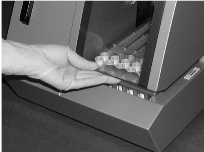
2. Rest the door on the door lock that is located near the top of the BioRobot EZ1 DSP.
