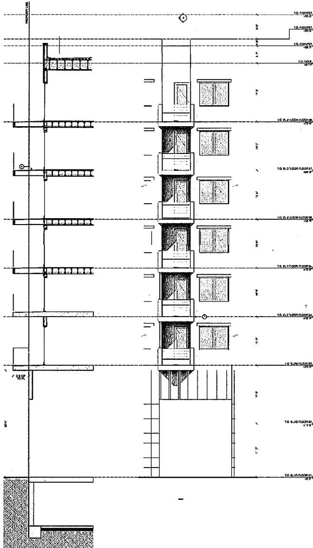
CONDITION 01 ELEVATION & WALL SECTION 4
