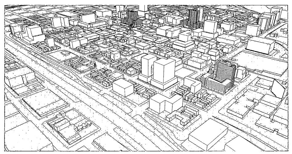
Note: This illustrative view is of building massing only (not design), as originally developed in August 2011. Existing buildings are shown in grey, new buildings are shown in white; and colored buildings are full-block concepts studied in greater detail. The view illustrates only one possible outcome of new development. All drawings will be updated in the Draft Plan based on feedback received to date as well as through the formal review process.
