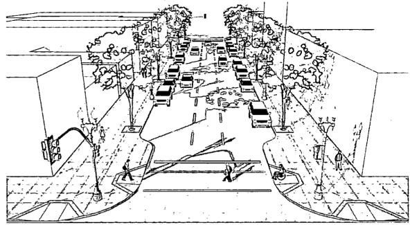
Phase 3 (Option A): Sidewalk Widening with Lane Reduction
