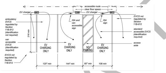
Figure 1- Specifications for ADA spaces and EV Charging Facilities from the Division of the State Architect
