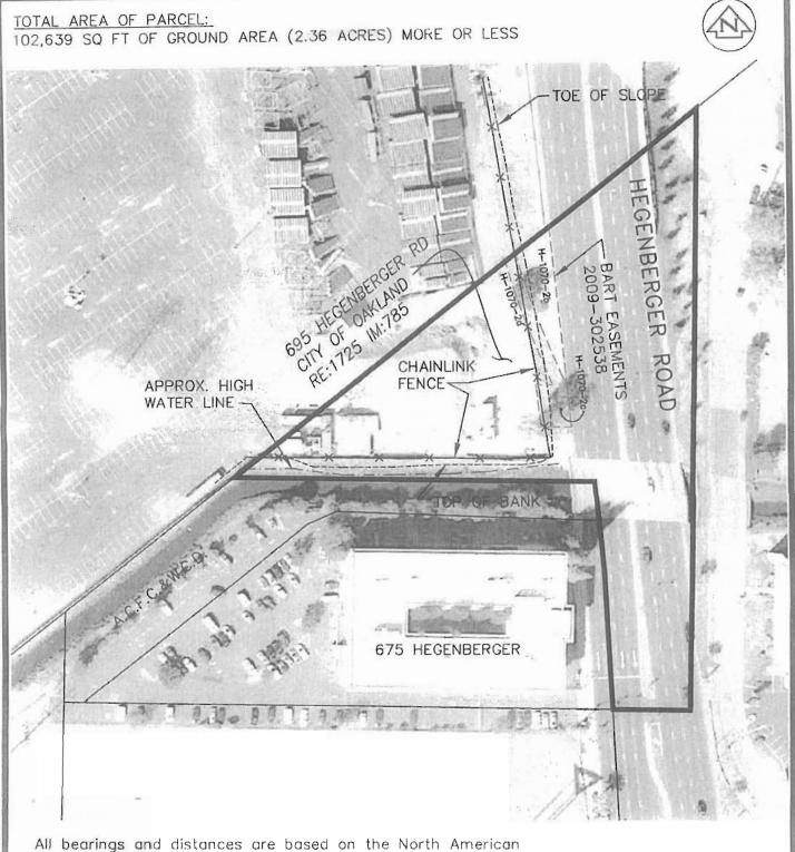
All bearings and distances are based on the North American Datum of 1983 (NAD83), Zone III. All distances are grid distances. To convert grid distances to ground distances, multiply expressed distances by 1.0000708.
