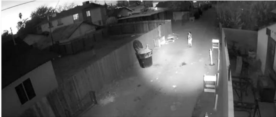
IR Floodlight: Infrared lighting will be used to enhance video image capture in low/poor lighting locations. The IR Floodlight can illuminate an area like a flood light that only the camera can detect.
