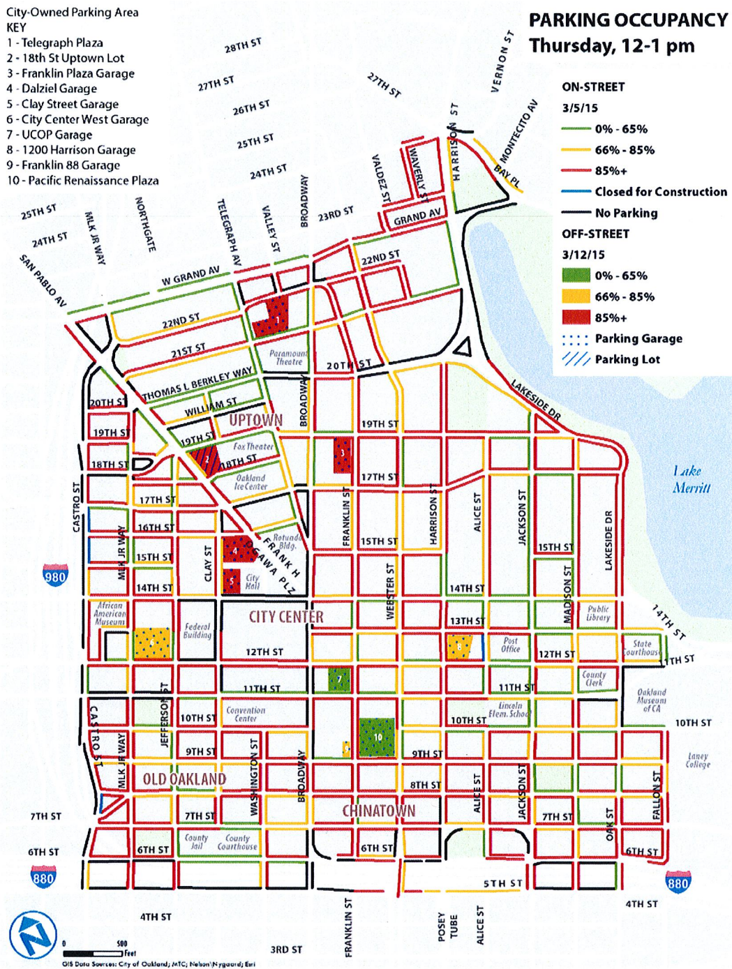
Figure 2-20 Parking Occupancy of Regular Spaces at Peak Hour (Thursday 12 p.m. to 1 p.m.)
