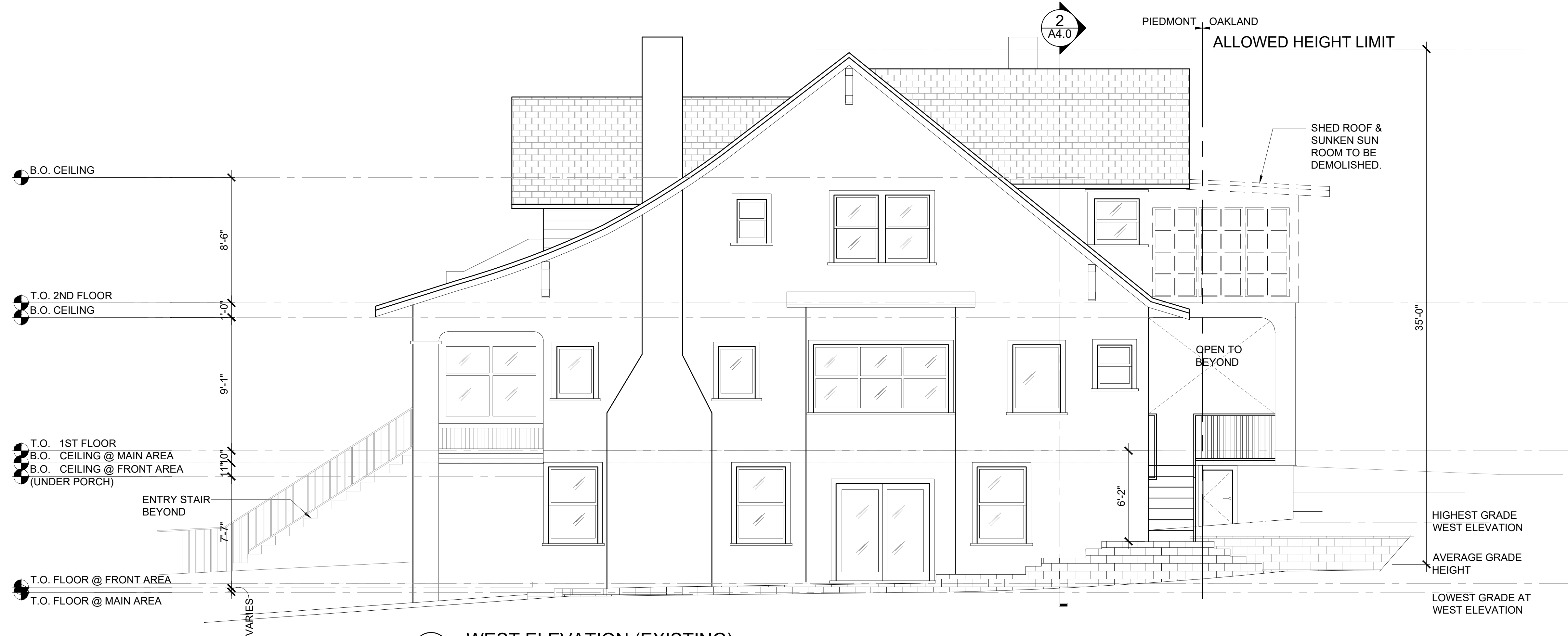
2 WEST ELEVATION (EXISTING)
