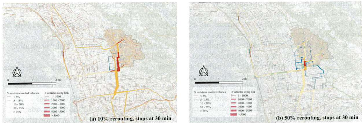
Figure 11. Total numbers of vehicles using each link (thickness) and percentages of vehicles with real-time rerouting on each link (color scale). (a) 15% of all evacuees follow real-time traffic information; (b) 50% of all evacuees follow real-time traffic information.
