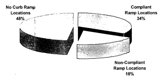
As of August 2008, the curb ramp database showed that about 5972 (34%) of a total of approximately 17,776 possible locations (street corners) have ADA compliant curb ramps. About 8,535 (48%) of possible locations have no curb ramp(s) and about 3,269 (18%) have non-compliant ramps.
