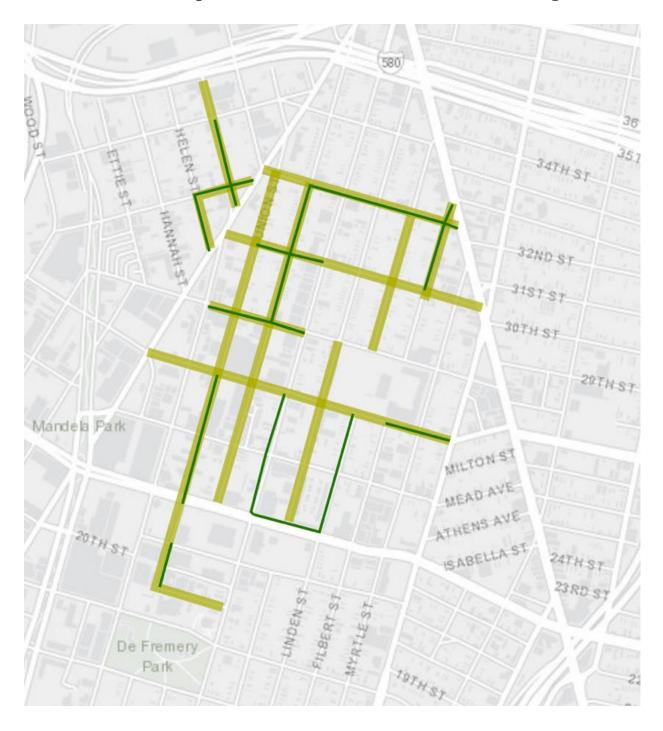
In the map above, the dark lines show EBMUD's pipeline replacement project. The light lines show the streets prioritized by the City for repaving under the 2019 3-Year Paving Plan.
