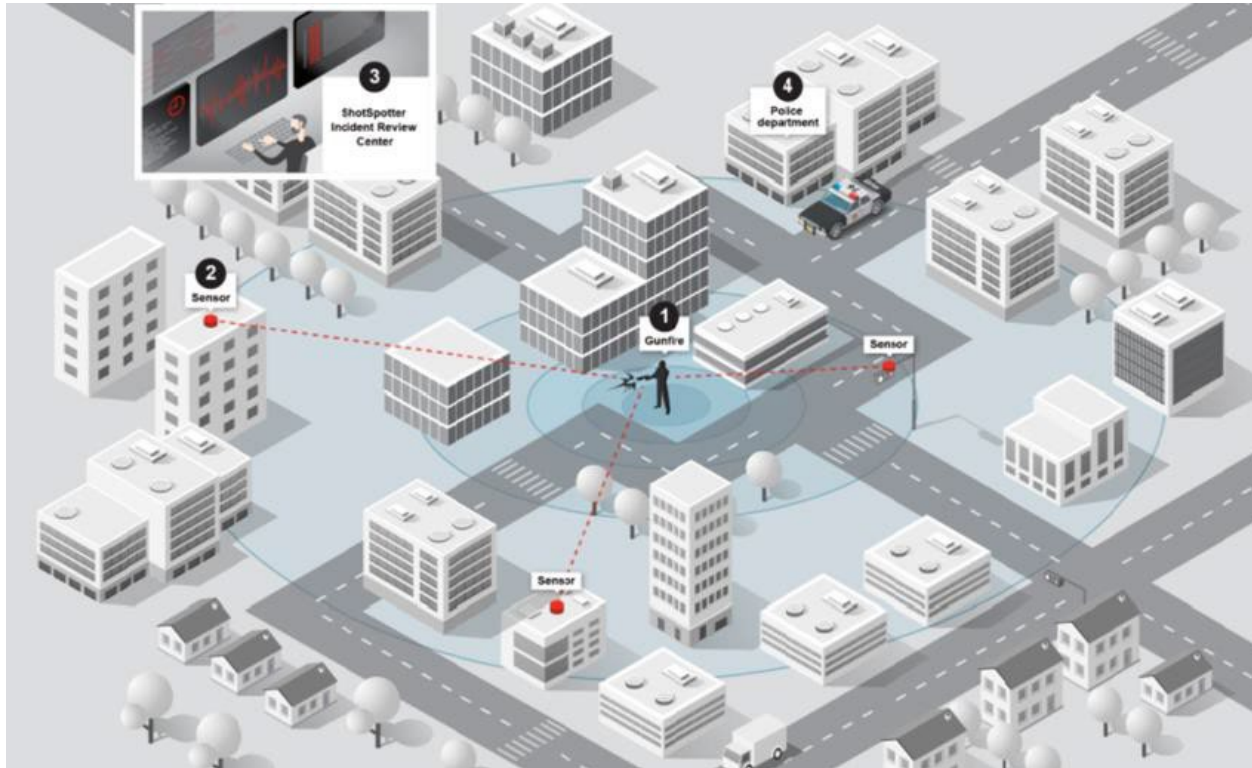
Figure 1 – How the ShotSpotter System Works
