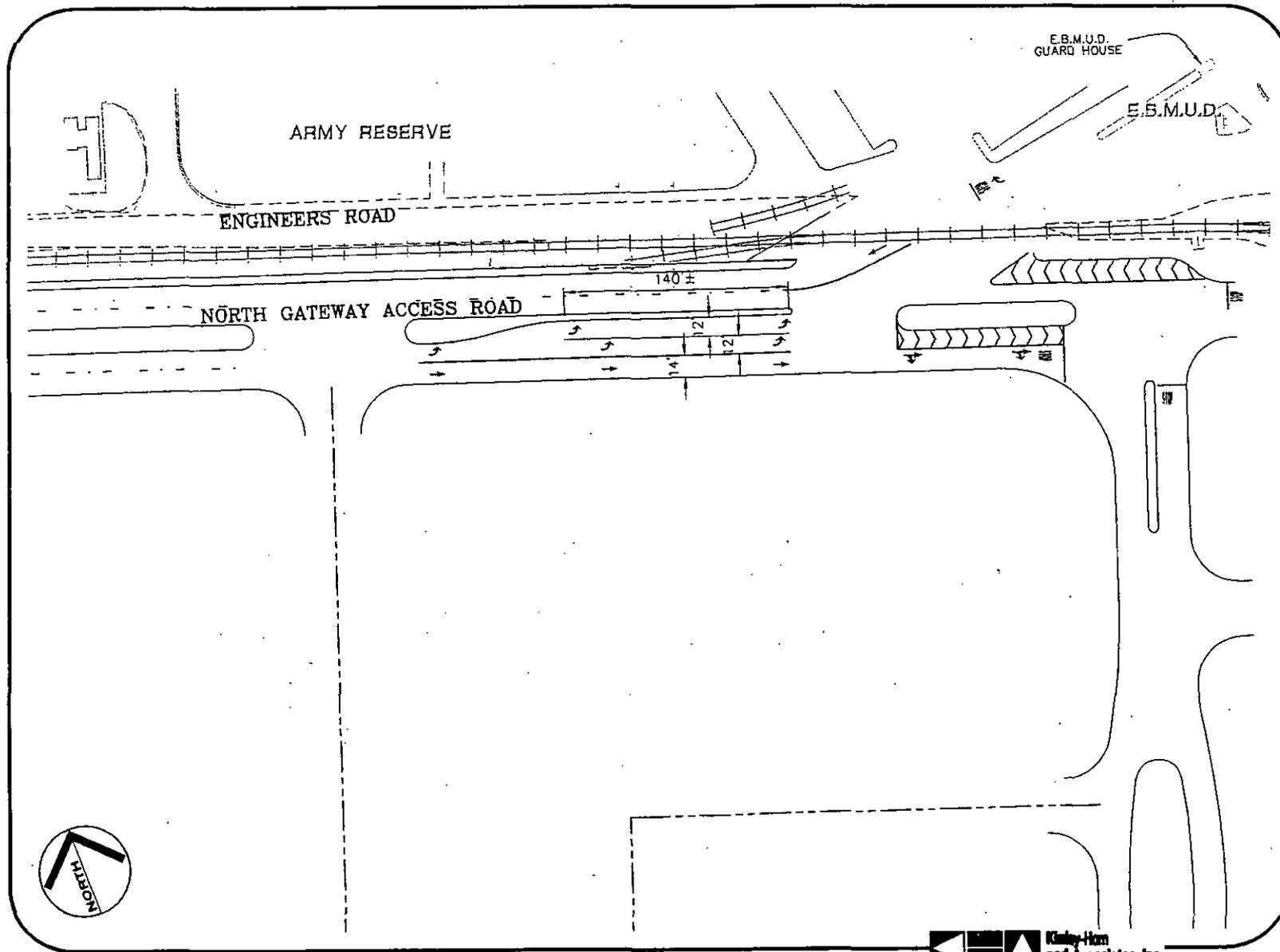
Figure 5: EBMUD Access - Left Turn Pocket Option
