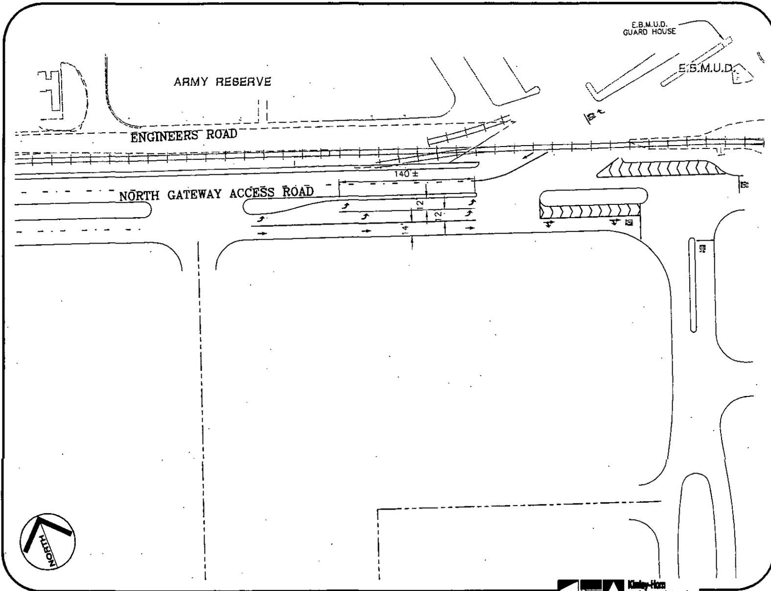
Figure 5: EBMUD Access - Left Turn Pocket Option
