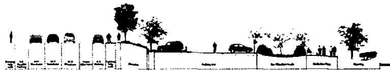
Section at Boathouse Parking and Bioswale
