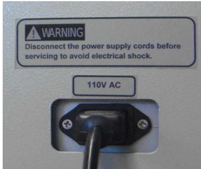
Figure 7-4 UV/HEPA power cable connection
