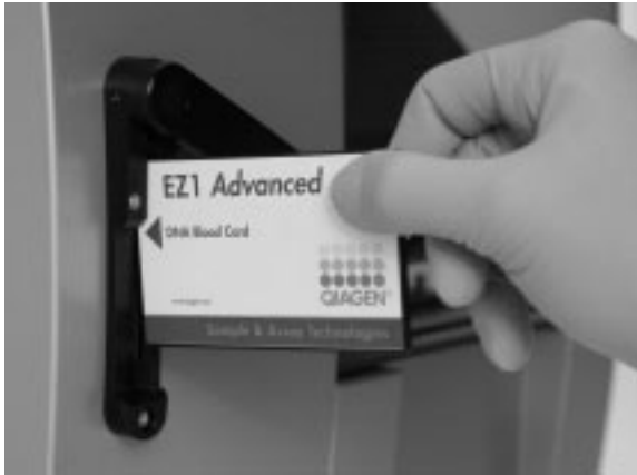
Figure 1. Ease of protocol setup using EZ1 Cards. Inserting an EZ1 Card, containing a protocol, into an EZ1 instrument. The instrument should only be switched on after an EZ1 Card is inserted. EZ1 Cards should not be exchanged while the instrument is switched on.
