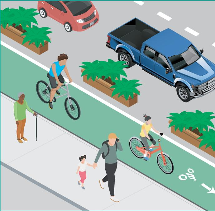
Figure 27. Cycle track protected by temporary planters. (Note: This specific design may not provide sufficient access to the curb.)
