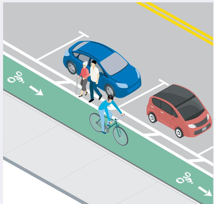
**Figure 19.** Parking-protected cycle track with narrow buffer and no accessible way of getting to the sidewalk.
