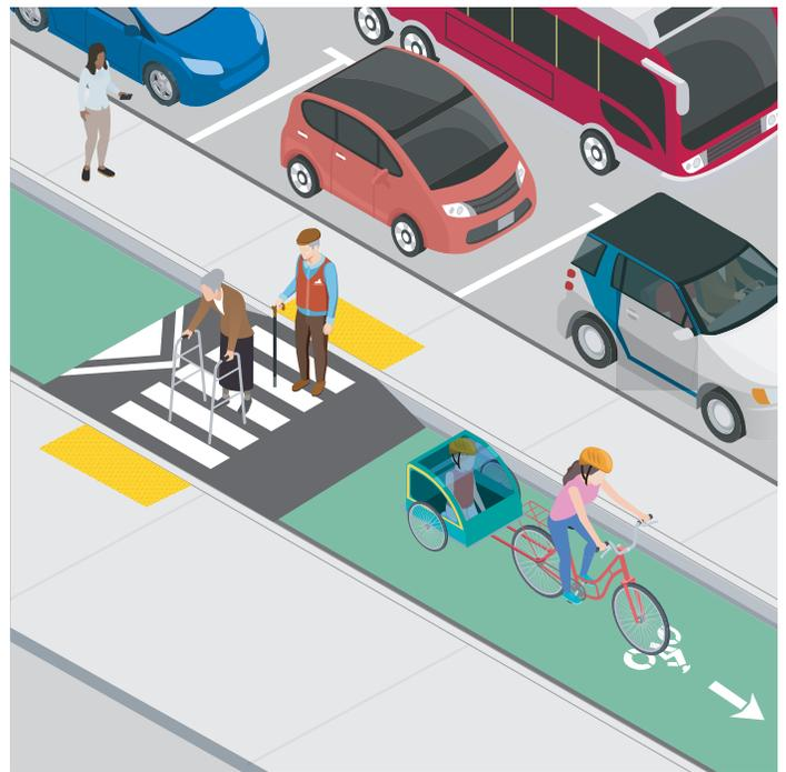
**Figure 10.** Cycle track protected by a concrete median, with a raised crossing. Median must be wide enough to comfortably navigate and facilitate wheelchair ramp deployment.
