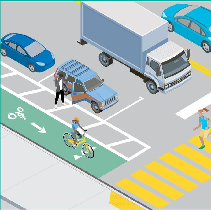
**Figure 22.** Parking-protected cycle track with ample buffer, free of obstructions, and leading to a crosswalk with a ramp.
