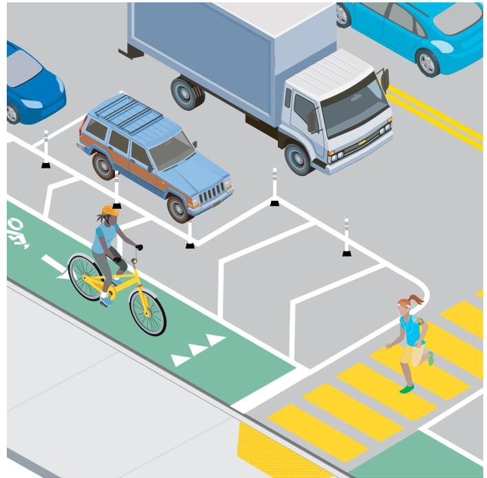
**Figure 20.** Parking-protected cycle track buffer area with confusing markings.
