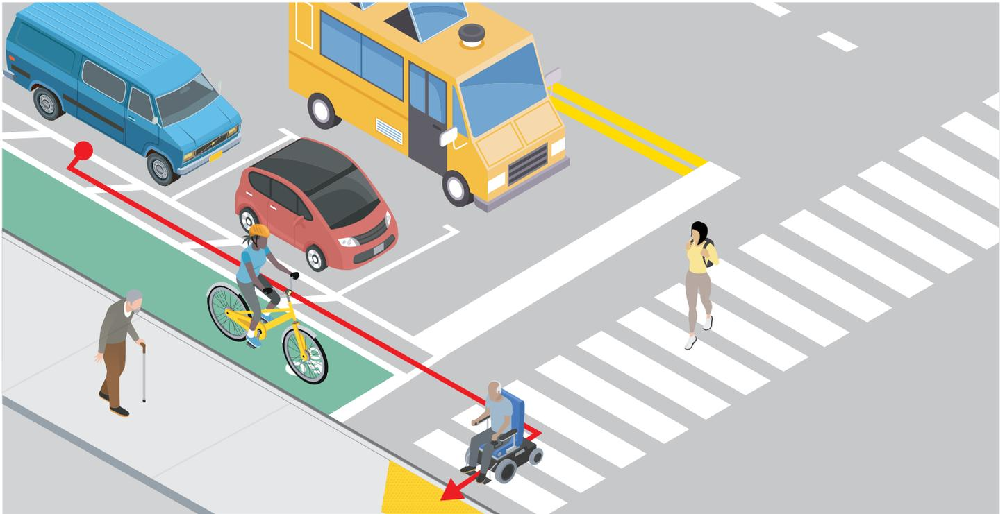
**Figure 9.** The arrow shows the path a person with a wheelchair, walker, or other assistive device must now travel to access the sidewalk from a parking spot that is located on the street-side of a cycle track.
