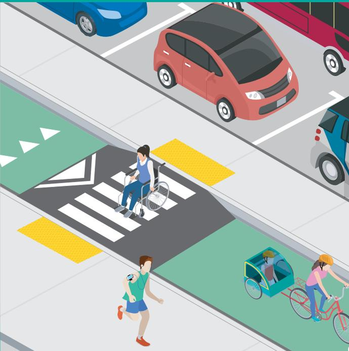
**Figure 24.** Parking-protected cycle track with a raised, wide median that serves as a buffer. Features a raised, high-visibility crossing from the buffer to the sidewalk.
