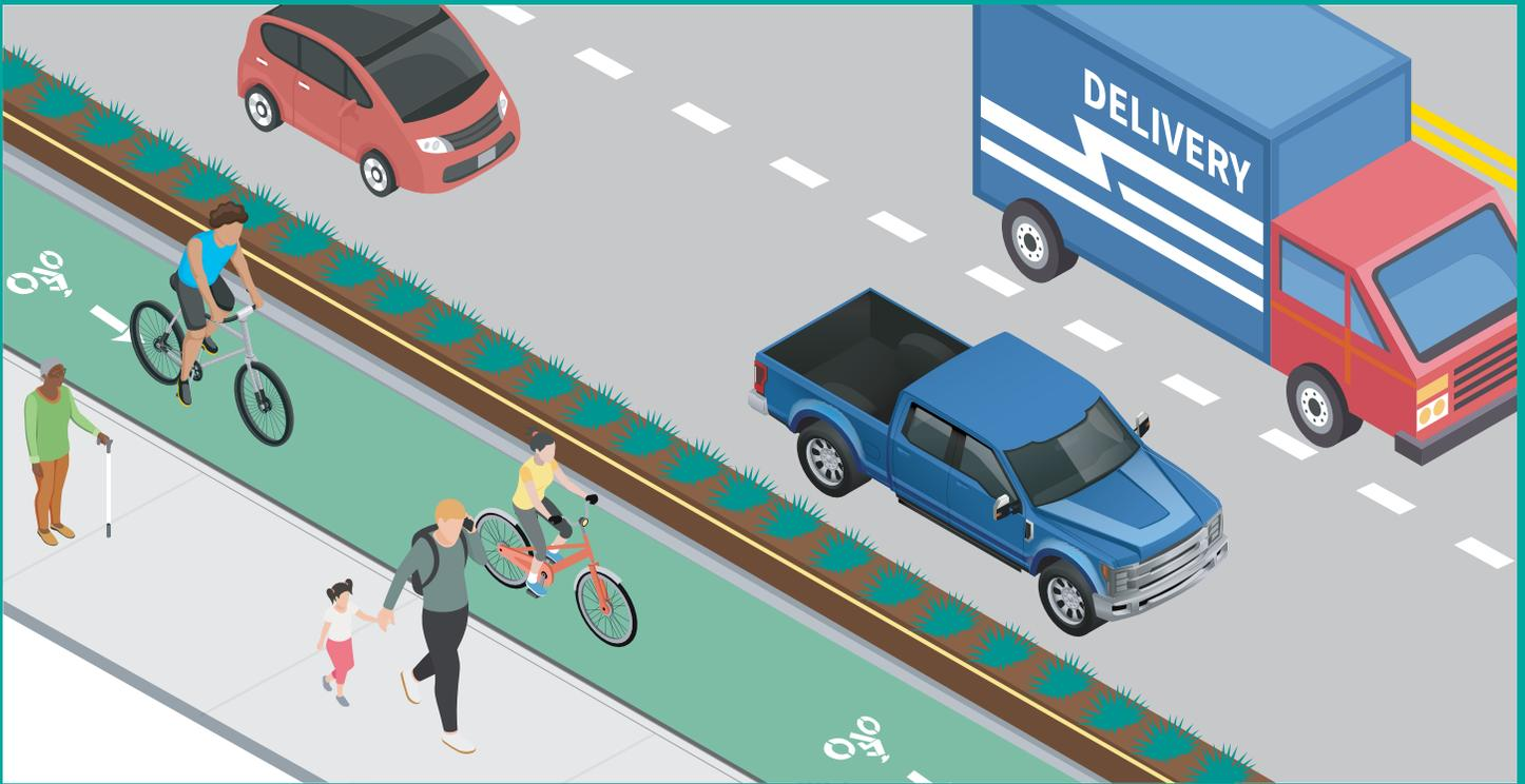
**Figure 7.** Cycle track protected by planters does not allow for accessible loading and unloading or paratransit pick-ups or drop-offs to destinations along the corridor.
