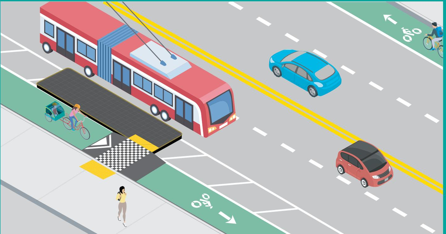
Figure 29. Pre-fabricated transit island that includes a raised cycle track crossing along the sidewalk curb.
