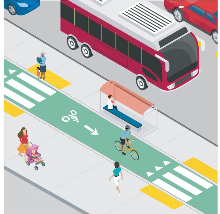
**Figure 15.** High-visibility raised cycle track with high-contrast crosswalks that lead to a transit island.
