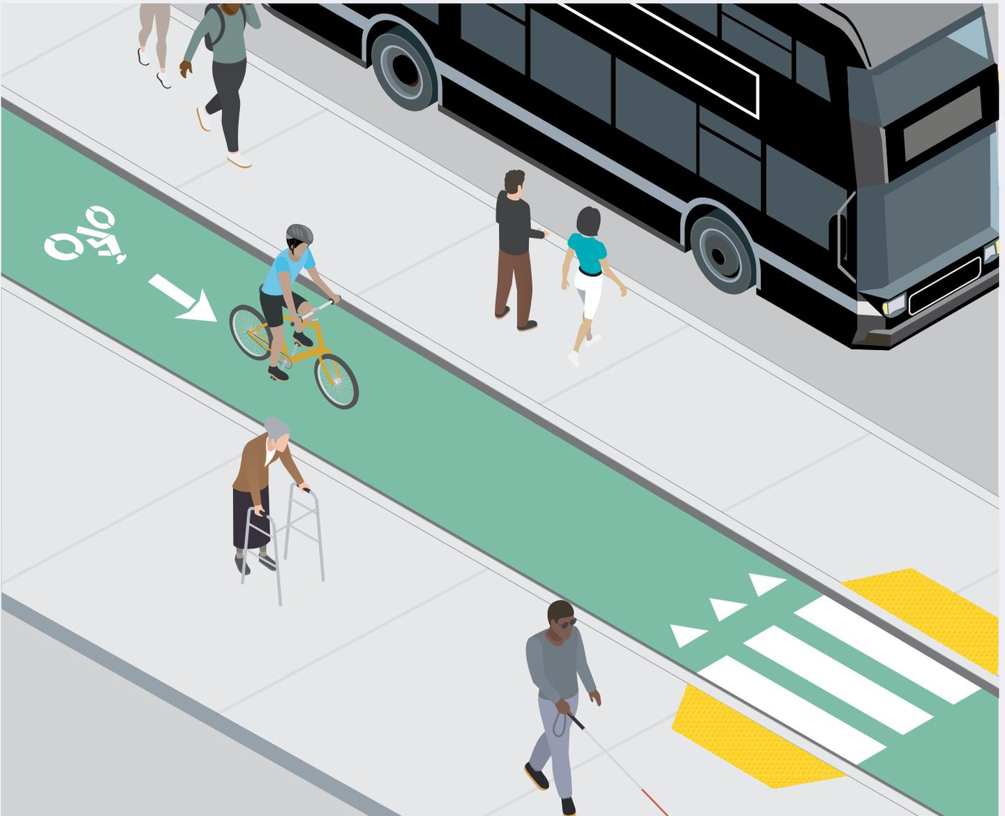
**Figure 16.** A shuttle picking up passengers from an accessible loading island.
