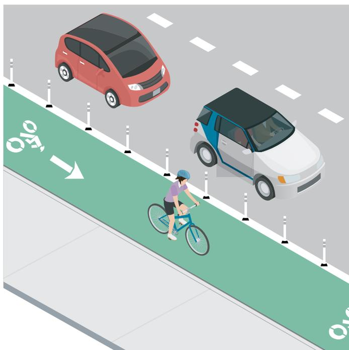
Figure 1. Cycle track protected by soft-hit posts.
