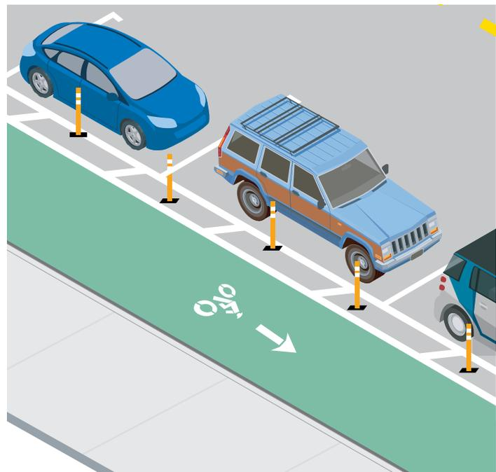
**Figure 21.** Parking-protected cycle track with orange delineator posts blocking vehicle loading and unloading possibilities as well as obstructing the buffer/path of travel area.
