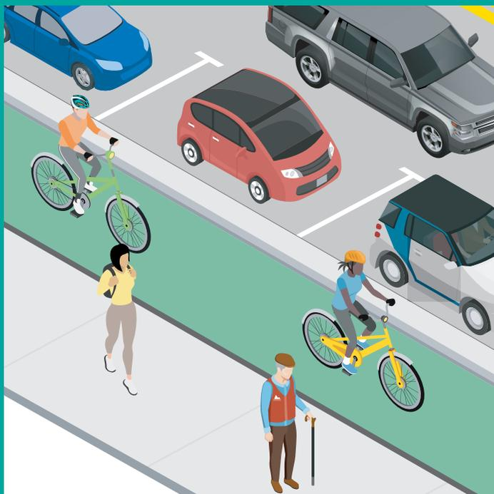
**Figure 5.** Cycle track protected by an inaccessible raised cement buffer. This buffer is too narrow for a person in a wheelchair or walker to navigate. It does not provide space for deployment of a vehicle wheelchair ramp. It also requires someone to dismount the raised buffer or travel to the end of the buffer zone to find a ramp.
