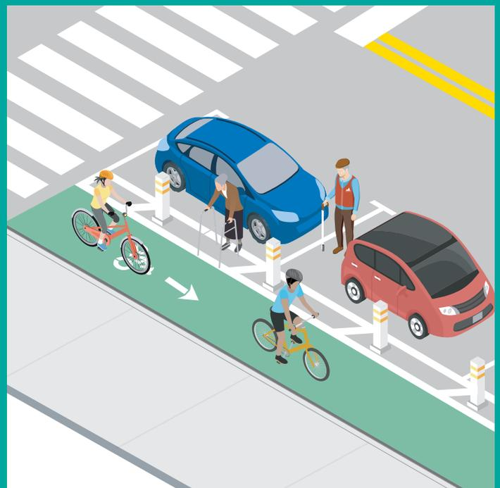
**Figure 6.** Parking-protected cycle track with no ability for people exiting cars to access the curb. Plastic bollards obstruct the "path of travel," forcing those who must access the sidewalk via a ramp to travel in the bike lane.
