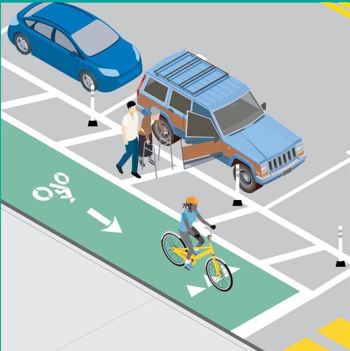
**Figure 25.** Parking-protected cycle track with soft-hit posts. Posts are spaced with enough room for vehicle doors to fully open and lifts or ramps to be deployed.
