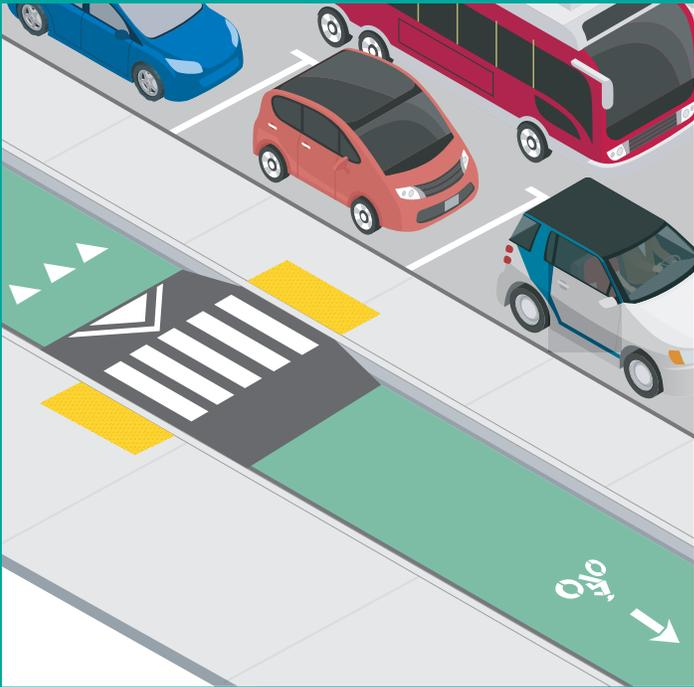
**Figure 23.** Parking-protected cycle track with a wide, unobstructed concrete median.
