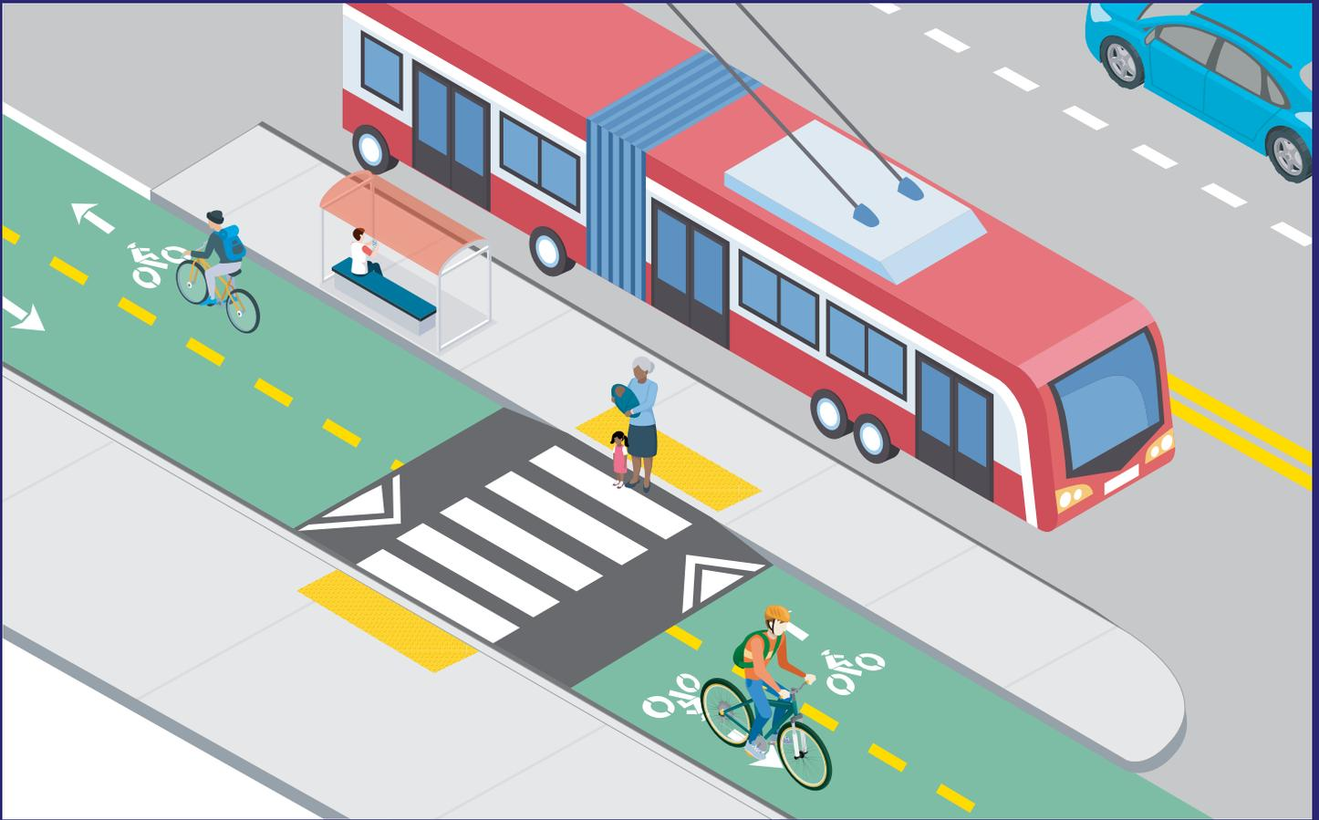
Figure 11. Two-way protected cycle track with a wide raised crossing to a transit island.
