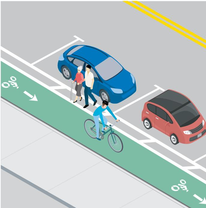
**Figure 8.** Parking-protected cycle track where two individuals have exited their car into a narrow buffer and are narrowly avoiding a cyclist passing by. There is no accessible way to reach the sidewalk once they cross the bike lane.
