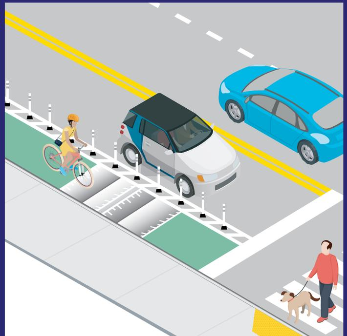
Figure 13. Speed bumps with drainage strips.
