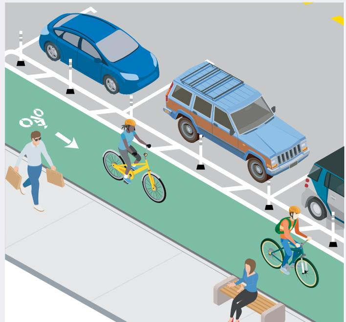
**Figure 18.** Parking-protected cycle track with narrow buffer and soft-hit posts obstructing the path of travel. A wheelchair user would not be able to unload from a vehicle in this design, and people using wheelchairs or walkers could not navigate safely down the buffer to an accessible crossing.
